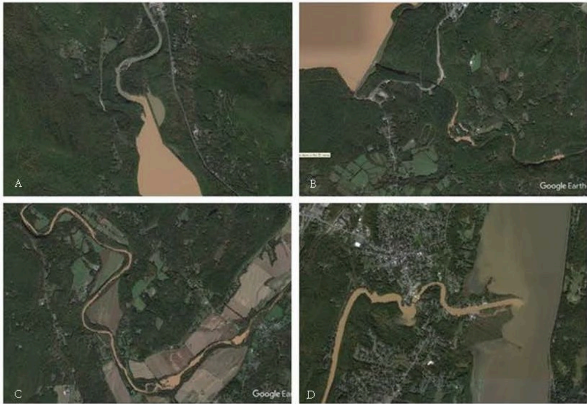
FIGURE 3: Aerial images of the Esopus Creek from October 2011 showing effects of reservoir releases on turbidity after a large rainfall event. From upper left (A), the upper Esopus can be seen entering the reservoir where it has started to return to a lower level of turbidity after a large event, seen as clear water entering the highly turbid reservoir. From upper right (B), the release from the reservoir can be seen entering the Lower Esopus channel. From lower left (C), the turbid water can be seen along the length of lower reaches including the Hurley Flats and that other tributaries are not contributing highly turbid water. From lower right (D), finally, the highly turbid water can be traced all the way to the Hudson River where it can be seen creating a turbid plume, in this case flowing up-river with the rising tide. All images oriented north with approximately equal scale; source: Google Earth.
