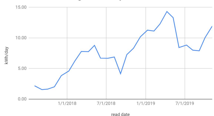
Comm Center EV Charger - kWh/day vs. meter read date
